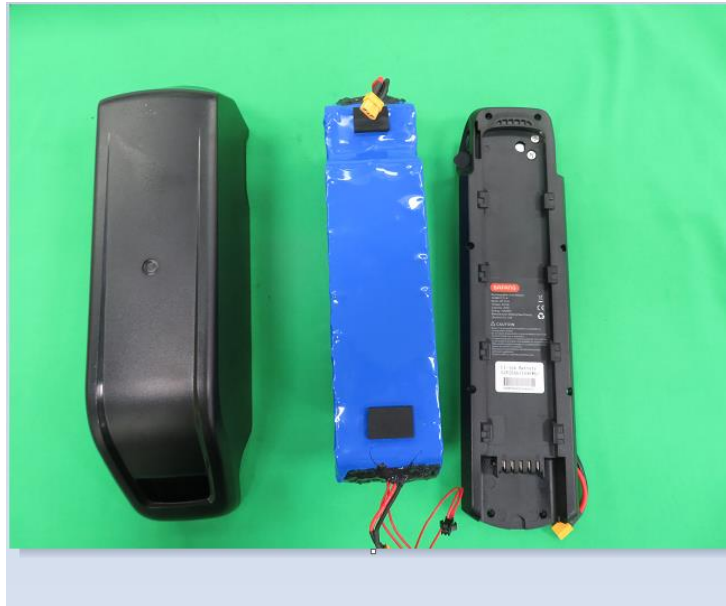
Internal view of battery BT F331
