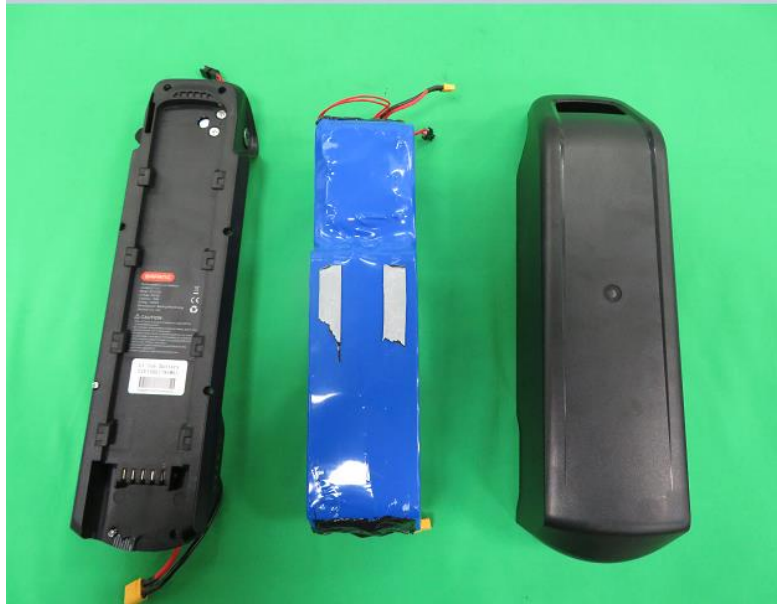
Internal view of battery BT F332
